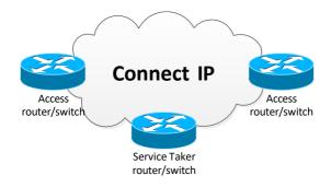
Connect IP is the location within TELE-POST's core network that connects all services provided to a Service Taker within a city or settlement with PoP connectivity. It may consist of a single router or of a city wide network made up of routers, switches and fiber interconnections.
