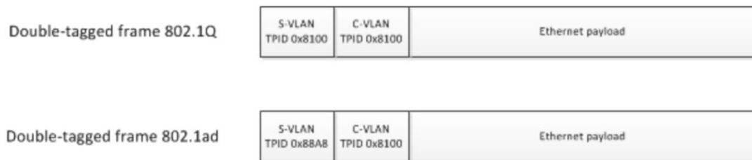
Figure 1 – S-VLAN tags on sub-interfaces
