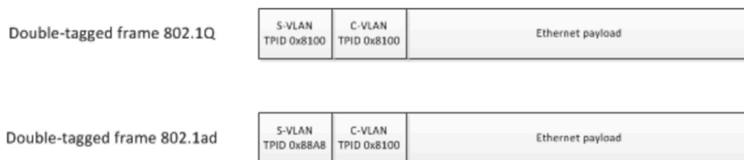
Figure 1 – S-VLAN tags on sub-interfaces
